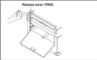
2. Move the release lever at the top left side to the FREE position (up direction).
